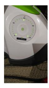
When the mini-USB is connected and the machine has power you will see these 3 lights
